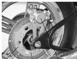
wear mark brake disc brake calipers
