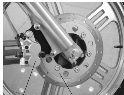
(Right) Brake calipers
